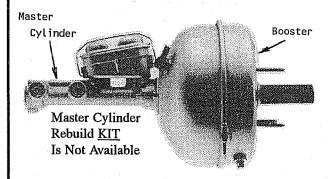
LK2021 Rebuilt Master Cylinder Only
