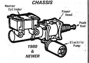
LK2809 New Power Head LK2814 Rebuilt Power Head
