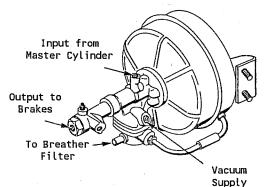
LK2001 New Booster LK2013 Rebuilt Booster
