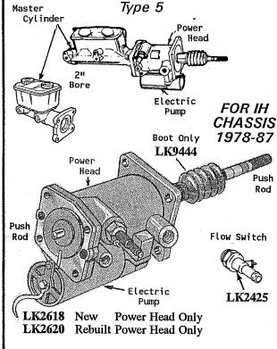
LK2418 New Electric Pump Only LK2420 Rebuilt Electric Pump Only
